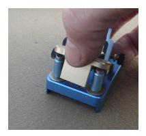
Turn the paddle over & thread the  $6-32 \times 1/2$  pan screws thru the holes in the base into the pin retainer. Note that one hole has a spot face in the anodize; this is for ground connection. Tighten both screws.
