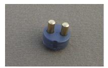
Now turn the insulator over & insert the two 4-40 x 3/16 screws with the #4 terminal lugs into the holes in the bottom of the insulator and thread them into the contact posts. Tuck the contacts together and snug the screws enough to hold the terminals in place. The contacts are pointing away from the notch milled into the edge of the insulator.
