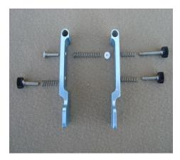
You are ready for the final assembly now. The 1/2'' thumbscrews should be threaded into the lever just a few turns, leaving plenty of clearance to install the levers. Slide each lever over it's dowel pin (finger paddles extended downwards). The lever fits between the stop pin & the contact post.
