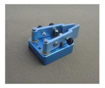
The spring sits tucked in between the levers close to the pin retainer; now is the time to install it while there is room for your fingers. Slide one end over the 7/16 pan screw in the left lever & the other end over the adjuster screw up against the Delrin washer.
