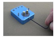
Turn the base over and loosen the 4-40 screws holding the terminal lugs, and spread the lugs apart & retighten. The posts may bind and tighten, or you may need to hold them. Turn the base on edge & hold the post with needle nose pliers while tightening the screws with a Philips screwdriver. You can put tape on the jaws to protect the brass, or simply use care.
