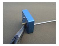
Turn the base right side up & slide the dowel pins into the bores in the base. Locate the two 3/16 washers; note that each washer has one side with rounded edges & one with rather sharp edges. Slide a washer over each dowel pin with the sharp edges
